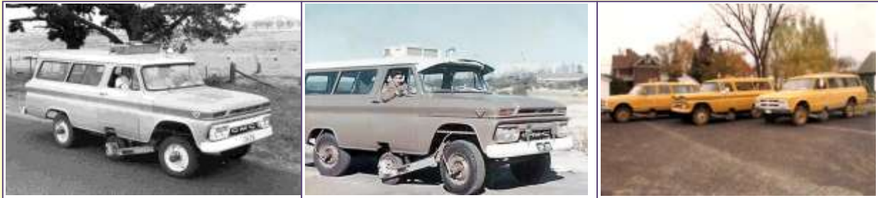
(Johnson) Ground Elevation Meters (L-R) : National Mapping, Royal Australian Survey Corps, United States Geological Survey (missing is a photo of the Canadian vehicle)
