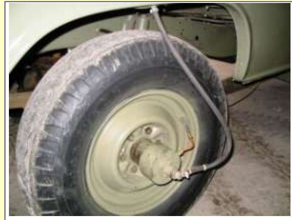
RASvy's JGEM showing tyre auto inflation fittings
