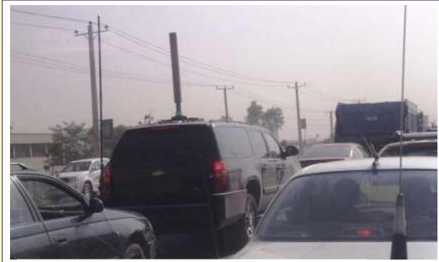
*Typical US Army vehicle in Kabul. The tall electronic jamming device on the roof stops all mobile phone reception in the area as they pass by.*
